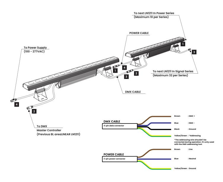
\*All devices in a DMX512 system must be connected in a "daisy chain" fashion. It is not permissible to have branching or splitting runs.
