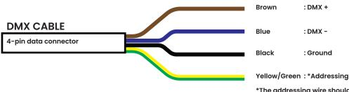
\*The addressing wire shouldn't be connected during operation. It's only used with the DMX addressing tool.
