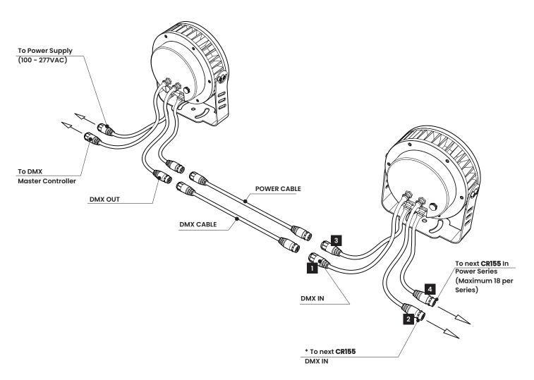
\*All devices in a DMX512 system must be connected in a "daisy chain" fashion.
