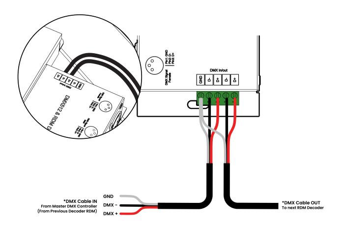
\*All devices in a DMX512 system must be connected in a "daisy chain" fashion.
