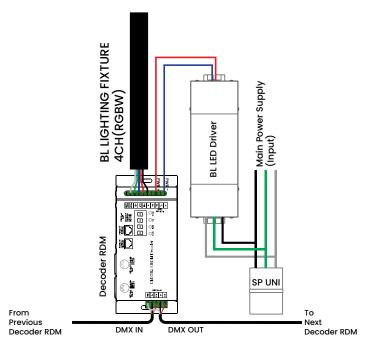
\*Ground wires(GND) must loop to each decoder
