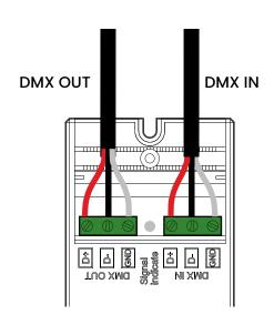
After each 10 decoders, an amplifier should be added to the daisy chain to maintain DMX signal quality.
