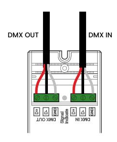
After each 10 decoders, an amplifier should be added to the daisy chain to maintain DMX signal quality.
