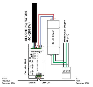
\*Ground wires(GND) must loop to each decoder
