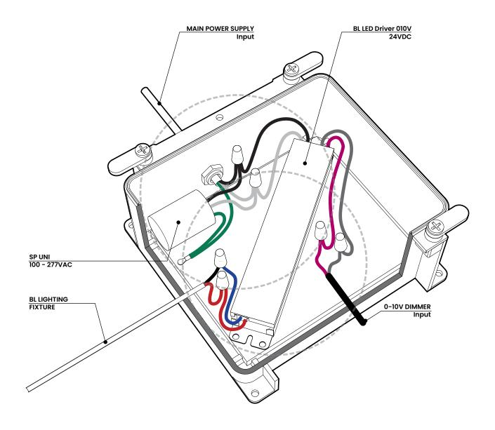
Follow the wiring diagram of a compatible dimmer instead, where applicable
