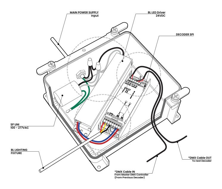
\*All devices in a DMX512 system must be connected in a "daisy chain" fashion.
