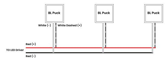
Connections 22 awg, 23.6" cable length, Parallel wiring
