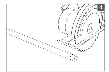
Use a Circular Saw to cleanly cut the clear Acrylic Tube.
