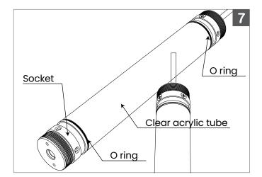
Slip the second O-ring over the end of the N360 light opposite the Lead Wire, and then secure the Socket to the other end of the **N360** light, as in Step 1.
