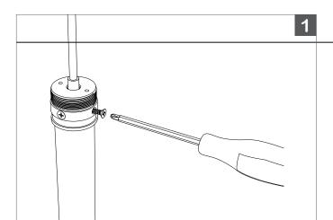
Route Lead Wire through Socket, and fully insert until it touches the end. Secure the Socket to N360 using (4) screws provided, and tighten until they are flush with the surface of the Socket.
