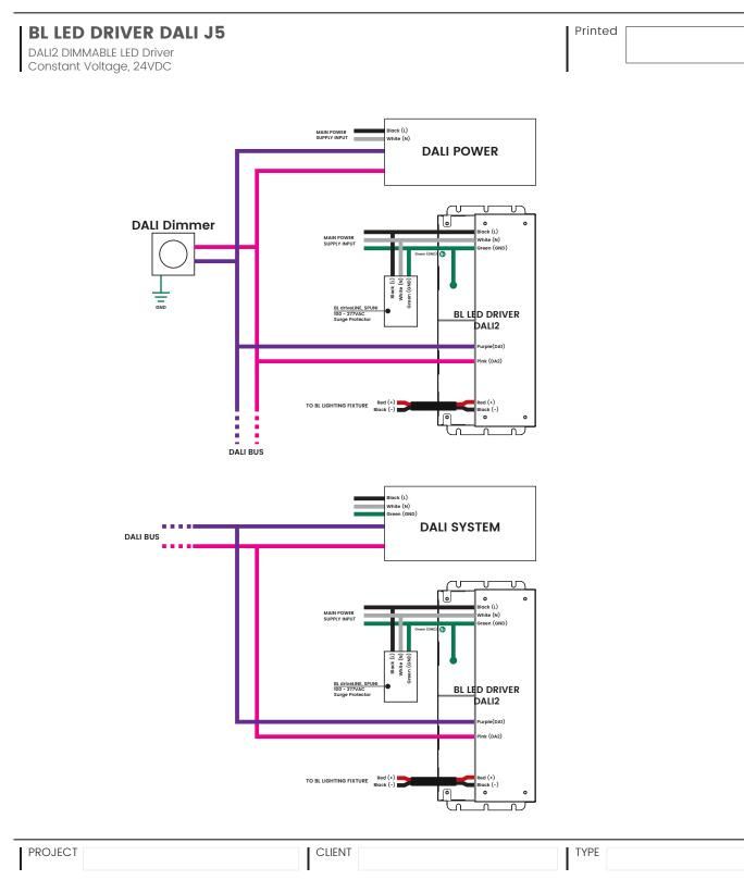
Solid State Lighting is sensitive to power fluctuations Surge protection is highly recommended for all LED lighting products and should be on a designated circuit to protect against premature failure Lack of surge protection may void your warranty
