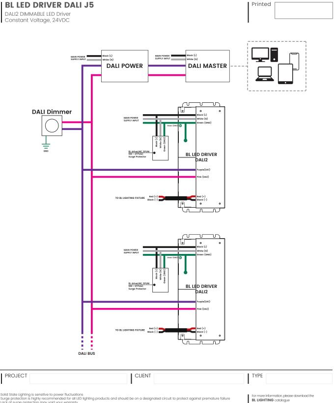
Solid State Lighting is sensitive to power fluctuations Surge protection is highly recommended for all LED lighting products and should be on a designated circuit to protect against premature failure Lack of surge protection may void your warranty
