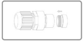
If applicable, connect fiber fitting to strain relief or bushing. Fiber fitting aligns fiber strands to the centre axis of light for maximum light acceptance.
