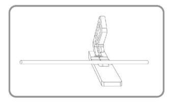
Fiber should be cut at 90° angle with a fiber cutter and with a sharp blade. A clean, clear cut will give maximum performance, whereas a cut with occlusions will result in light loss.
