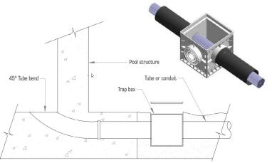
The 45° bend should be adjusted and cut to coincide with the pool floor and thus ensuring a gentle bend in the fiber access
