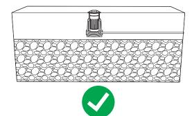
IK10 rated and designed to bear pressure loads up to 4409lbs (2000 kg) from vehicles with pneumatic tires. The luminaires must not be used for traffic lanes where they are subject to horizontal pressure form vehicles changing direction, acceleration or breaking.
