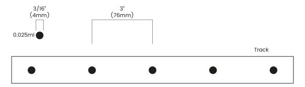
Place a small dab (0.025ml) of adhesive onto the inside ridge of the BL fixFORM base track channel at 3" intervals.
