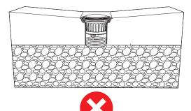
IK10 rated and designed to bear pressure loads up to 4409lbs (2000 kg) from vehicles with pneumatic tires. The luminaires must not be used for traffic lanes where they are subject to horizontal pressure form vehicles changing direction, acceleration or breaking.
