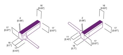
The tolerance of the Lead is ±0.5mm For more detail, please download the CAD Drawing
