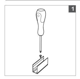
1. Arrange clips per installation requirements, and surface mount them with screws.
