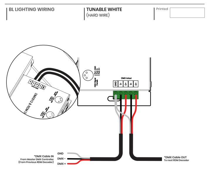
\*All devices in a DMX512 system must be connected in a "daisy chain" fashion.
