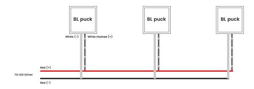
Connections 22 awg, 23.6" cable length, Parallel wiring
