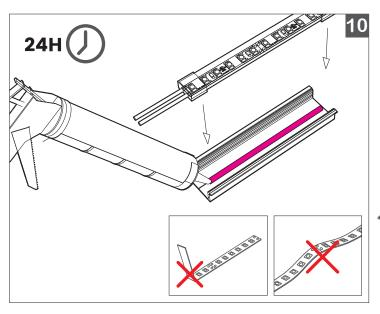
IMPORTANT: Allow adequate time for adhesive to cure, a minimum 24 hours is recommended. Refer to the instruction on the specific adhesive being used for guidance.
