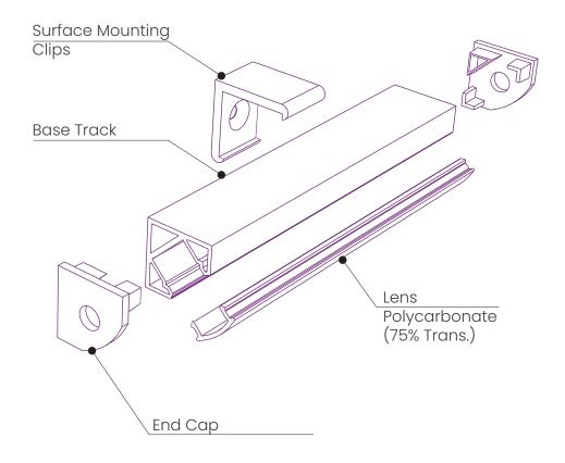
Each 6ft length of LED Profile is shipped complete with End Caps and Mounting Clips.
