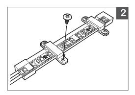
2. Mount clips to surface with screws.
