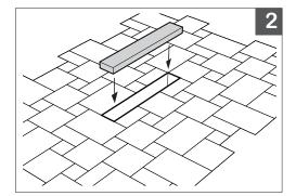
2. Insert foam base. Add or shave down foam base until optimal height is acheived for flush installation of RC65.
