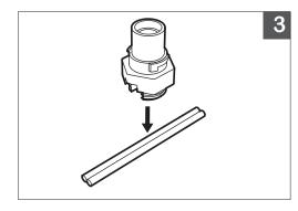
3. Secure Lamp Holder onto the Wire
