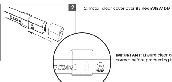
**IMPORTANT:** Ensure clear cover orientation is correct before proceeding to Step 3.
