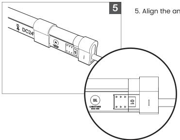
5. Align the anti-skid clips onto the power connector.
