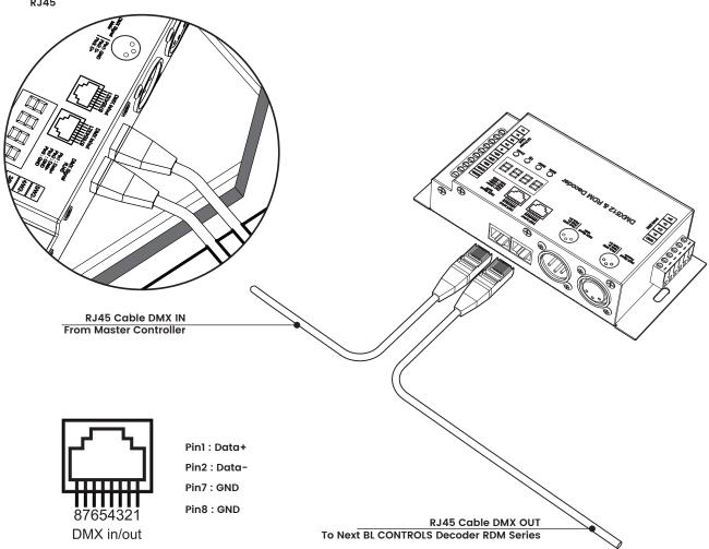
\*All devices in a DMX512 system must be connected in a "daisy chain" fashion.
