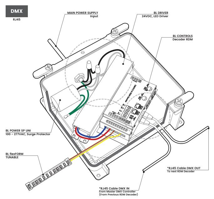
\*All devices in a DMX512 system must be connected in a "daisy chain" fashion.
