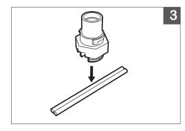
3. Secure Lamp Holder onto the Wire
