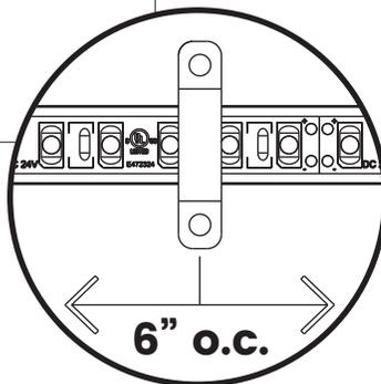
**NOTE:** Two clips per linear foot is recommended for secure fastening.
