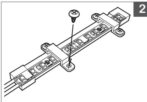
2. Mount clips to surface with screws.
