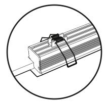
**TIP:** Minimum two Spring Clips per section recommended for secure fit behind drywall.
