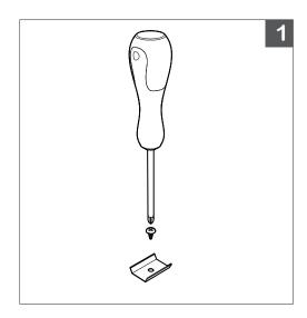
1. Mount clip to surface with screws.
