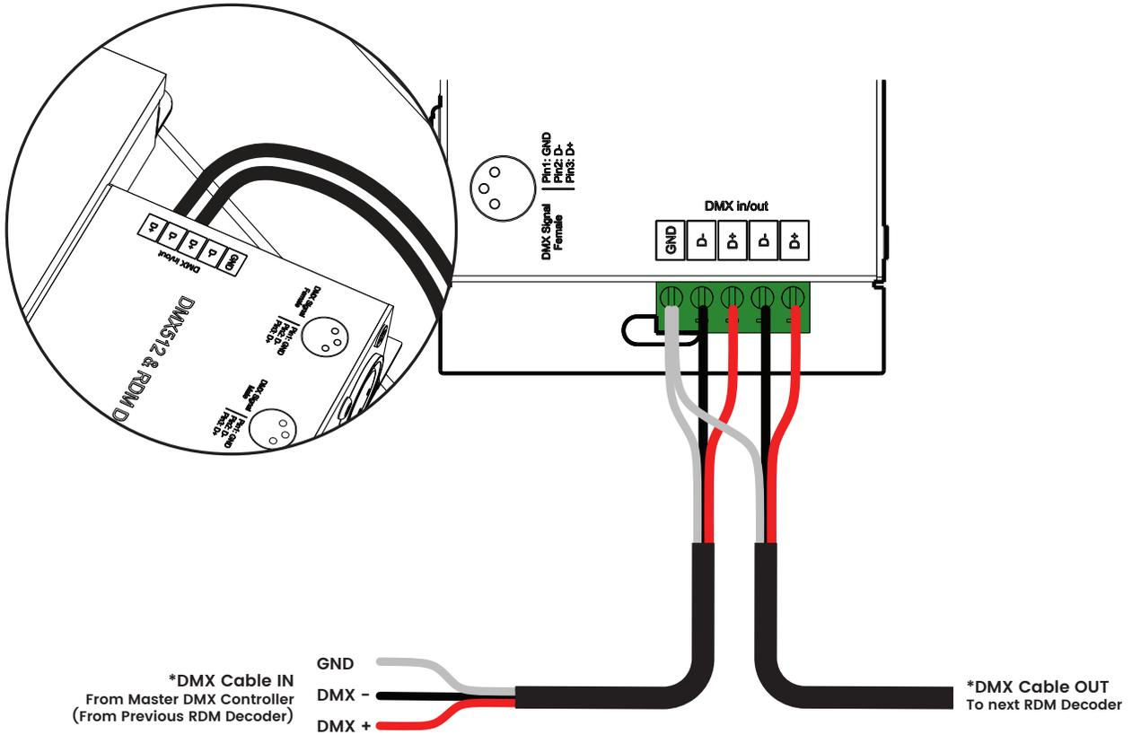
\*All devices in a DMX512 system must be connected in a "daisy chain" fashion.
