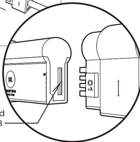
**TIP:** Copper located on right side of PCB
