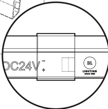
**IMPORTANT:** Ensure clear cover orientation is correct before proceeding to Step 3.
