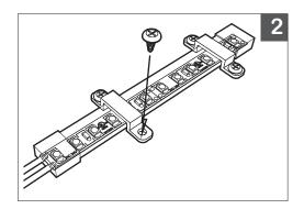
2. Mount clips to surface with screws.
