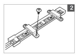
2. Mount clips to surface with screws.
