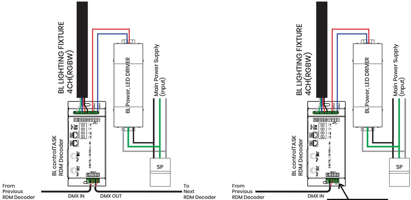
\*Ground wires(GND) must loop to each decoder
