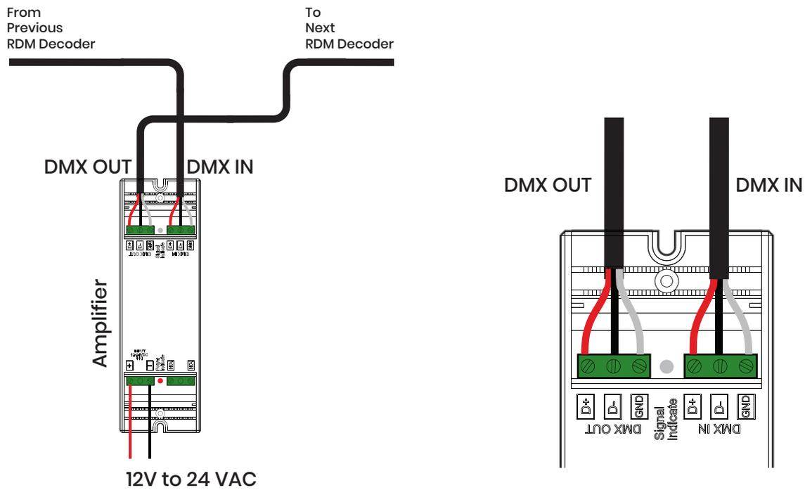
After each 10 decoders, an amplifier should be added to the daisy chain to maintain DMX signal quality.
